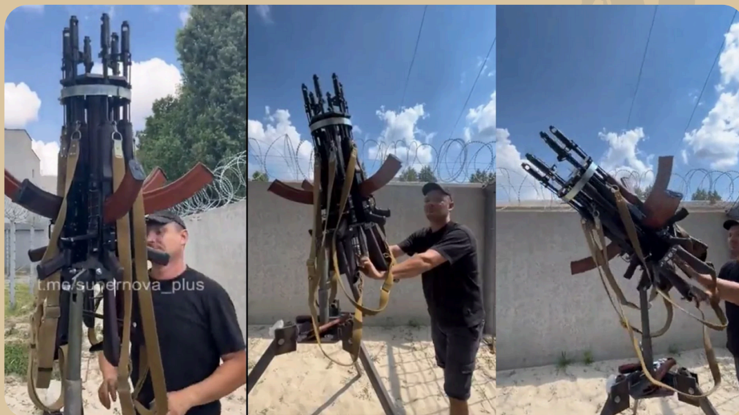
Improvised system consisting of six AK-74 rifles.
